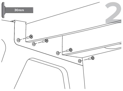
Secure the legs to the support using the 30mm bolts provided.
