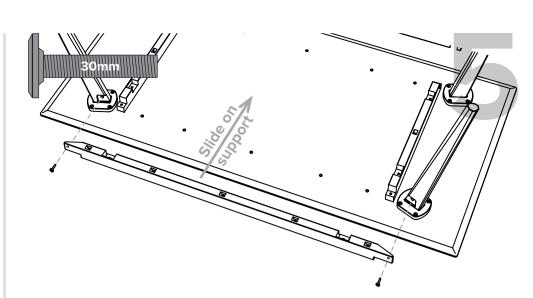
Slide the long supports into their corresponding slots in the legs and short supports. Secure the long supports to the legs using 30mm bolts.
