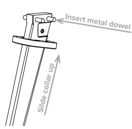
Slide a collar along the leg and insert a metal dowel into each of the holes at the top of the leg.
