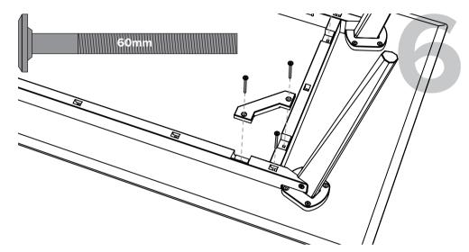
Slot the corner pieces into place in the long and short supports. Secure the corners, long & short supports using 60mm bolts.
