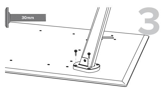
Put the legs in the pockets on the table top and loosely secure it in place with 30mm bolts. Once all four bolts are in, tighten each until they are firm using the allen key.
