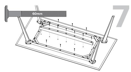
Insert remaining 60mm bolts into supports and check that everything is nice and tight. If you have a larger sized table, you will have an additional support (shown above). Fit this to the center of the table and secure using 60mm bolts.
