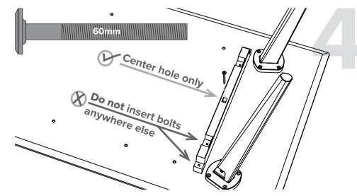
Place the short supports in position and loosely insert a 60mm bolt into the centre hole only.
